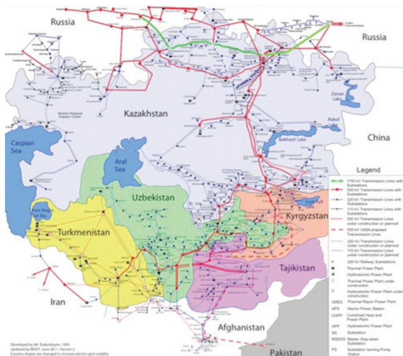
Figure 7. Central Asian (Electric) Power System.
